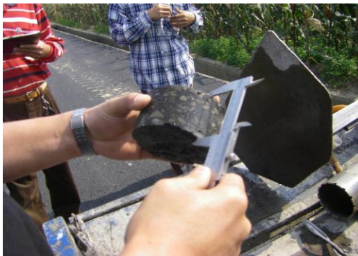
Measuring the thickness by vernier calipers
